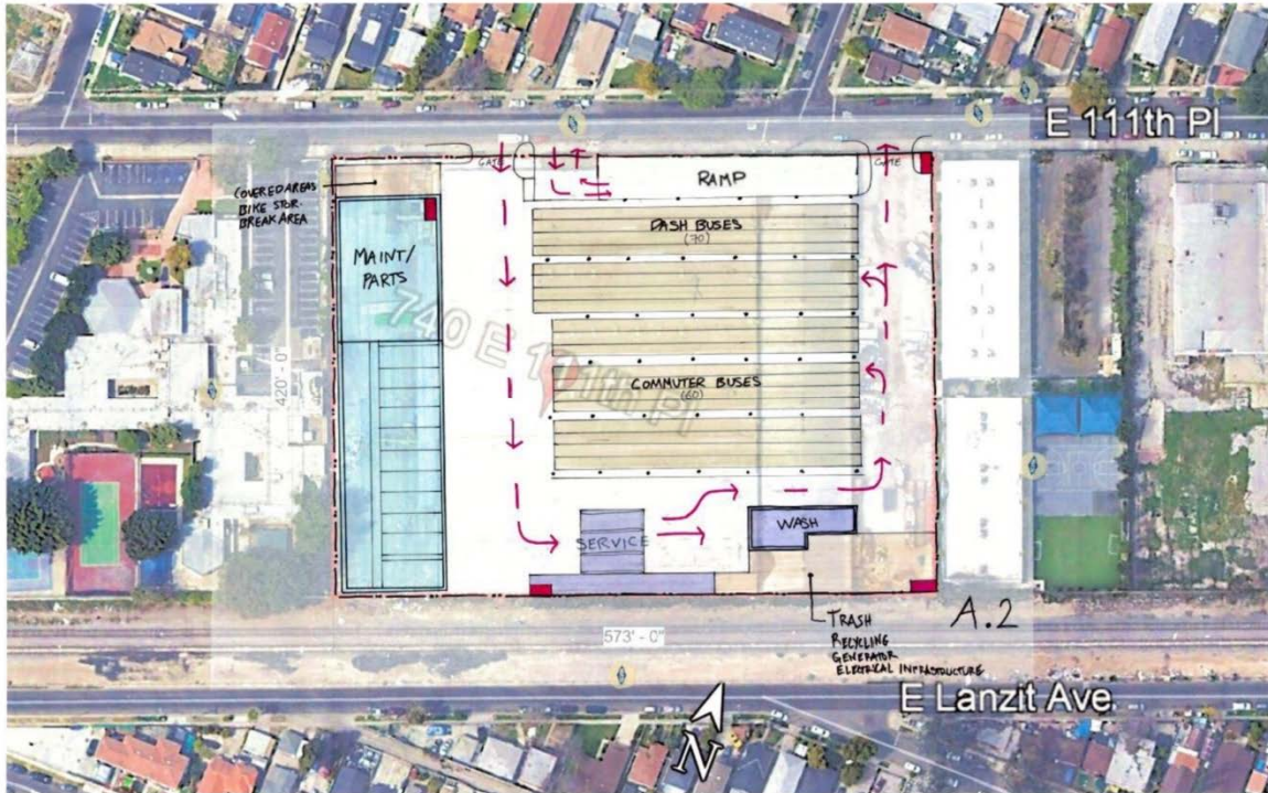
Figure 2-4: Conceptual Ground Level Floor Plan
